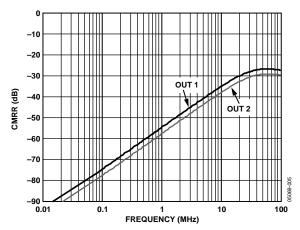
Figure 8. Common-Mode Rejection (CMRR) vs. Frequency ( $V_S = \pm 5$  V,  $R_L = 25$   $\Omega$ )
