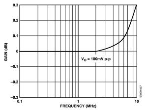
Figure 10. 0.1 dB Flatness  $(V_S = \pm 5 V, V_O = 0.1 V p-p, Gain = +1, R_L = 25 \Omega)$
