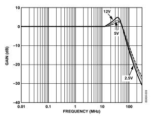
Figure 12. Small Signal Frequency Response for Various Supplies (Gain = +1,  $V_0 = 0.1 \text{ V } p$ -p,  $R_L = 25 \Omega$ )
