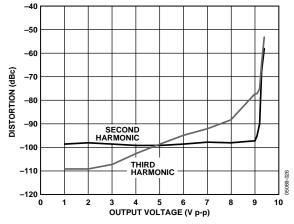
Figure 20. Distortion vs. Output Voltage @ 100 kHz,  $(V_S = \pm 5 V, G = +2, R_L = 25 \Omega)$
