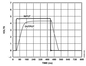
Figure 22. Unity-Gain Input Overdrive Recovery
