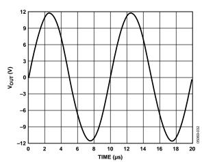
Figure 3. Output Swing,  $V_S = \pm 12 V$ ,  $R_L = 100 \Omega$
