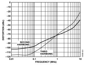
Figure 17. Distortion vs. Frequency  $(V_S = \pm 5 V, V_O = 2 V p-p, G = +2, R_L = 25 \Omega)$
