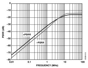
Figure 16. Power Supply Rejection Ratio (PSRR) vs. Frequency ( $V_S = \pm 5 \ V, R_L = 25 \ \Omega$ )
