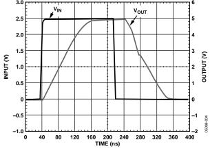
Figure 7. Output Overdrive Recovery  $(V_S = \pm 5 V, Gain = +2, R_L = 25 \Omega)$
